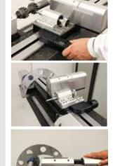
**GIOTTO-MAN** is a manual measuring bench for shafts designed to be placed in the production floor for an immediate feedback on the tolerance limits. Diameter and Length measurement axis are activated by operator. The repeatability is ensured by a dedicated mechanical system.
